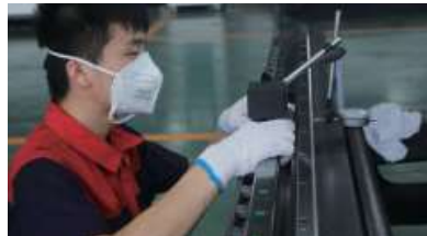
03 PARALLELISM INSPECTION Assembly and adjustment of rack parallelism accuracy.
